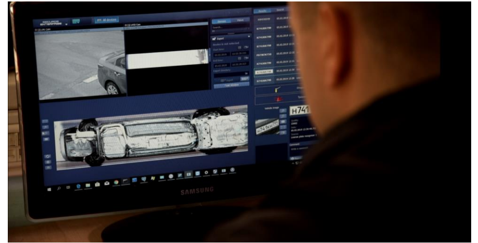
Automatically highlighting differences in current undercarriage image and reference image
